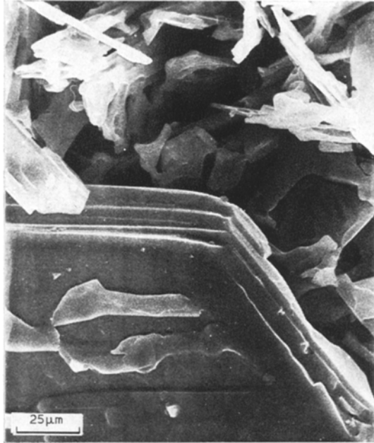
Figure 2 Scanning electron micrograph of growth front of extracted primary silicon showing multiple twin traces in Al-16 wt % Si alloy.
